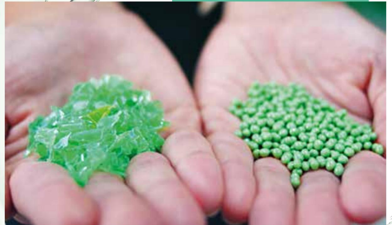
**Ice River had recently bought an XFORM preform injection molding system to process 100% post-consumer PET recycle into preforms for its 500-mL spring water bottles.**
