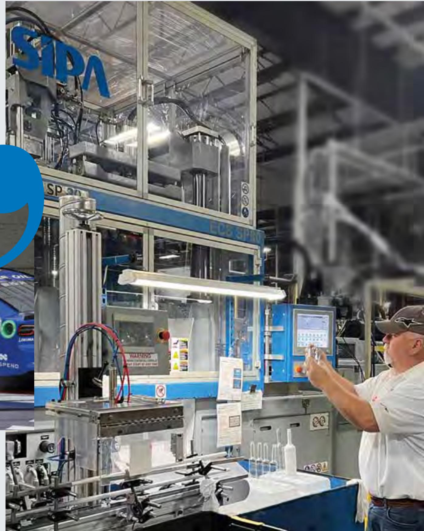
Single-stage production using the ECS SP 80 is ideal for these particular bottles, given the production numbers and the variety of sizes involved. The SIPA units run fast and efficiently, and the time and effort involved in changing format is low. The bottle maker can rely on responsive technical support from the people at SIPA North America, and that includes short turn-around times for any mold renovation or repairs.
