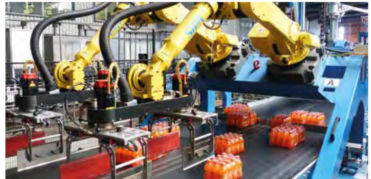
range of solutions for different container handling in plastic crates, American-type cartons and wraparound, designed to meet different levels of speed and to cover all production needs, from the simplest to the most complex packaging configurations handled with robotic solutions.
