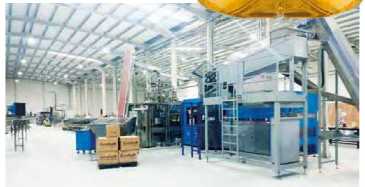
Also included in the package was a labelling unit, equipment for inserting handles into the bottles, and a SIPA PTF 1 palletizer. On top of all this, SIPA provided auxiliaries and the piping along the line. Everything is highly automated, with a supervisor carrying out monitoring and providing production reports.
