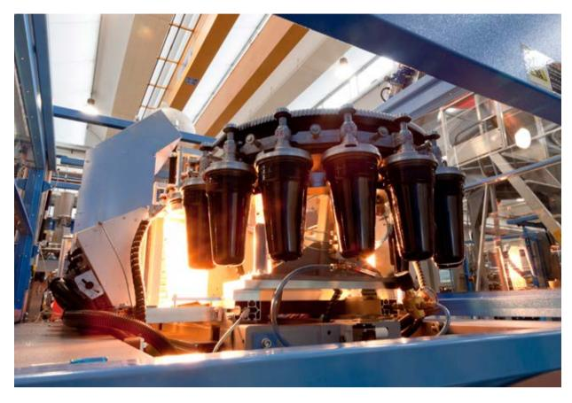
SIPA's very broad range of stretch-blow molding machines caters for diverse customer needs in terms of output rates and container size; there is of course also the choice between linear and rotary machines. One especially versatile model is the linear SFL 4/3 XL, with its ability to hold one, two, or three cavities (format changes are quick and simple to carry out) and to produce containers as small as 12 mL and as large as 12L, at speeds of up to 5400 bottles per hour.
