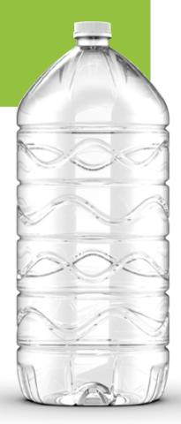
This means that, when switching formats. time is needed not only to change the mold for the bottle body, but also for the neck. Using a 38-mm neck for both formats takes care of that issue. Plus, preforms with a 38-mm neck are lighter - around 6g lighter - than preforms with 48-mm necks, lower in cost, and more available. On top of that, caps for the narrower neck are easier to find on the market.
